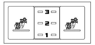
Your vehicle may have this feature. The buttons used to control the heated rear seats are located on the back of the center console. The engine must be running for the heated seat feature to work.
